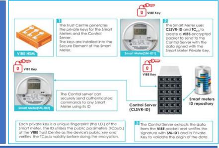
A sample setup of a smart meter communication within a BAS environment is shown. The VIBE protected deployment is set up, and then taken offline, effectively eliminating threats from "online" attackers.
