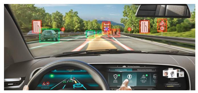
A system for low-speed application which is activated by the driver and which keeps the vehicle within its lane for travelling speed of 60kph or less by controlling the lateral and longitudinal movements of the vehicle for extended periods without the need for further driver input
