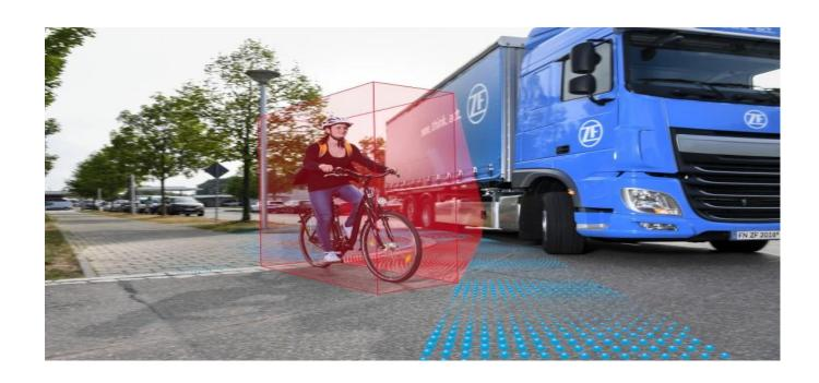
Blind-spot monitoring uses a set of sensors mounted on the side mirrors or rear bumper to detect vehicles in the adjacent lanes. If the sensors detect something, they'll alert you via an audible and/or visual warning. Some vehicles even use a camera as the main part of the system or to complement the sensors.
