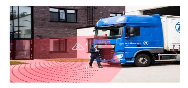
A system used to detect and inform the driver of the presence of pedestrians and cyclists in the close-proximity forward blind-spot of the vehicle and, if deemed necessary based on manufacturer strategy, warn the driver of a potential collision.
