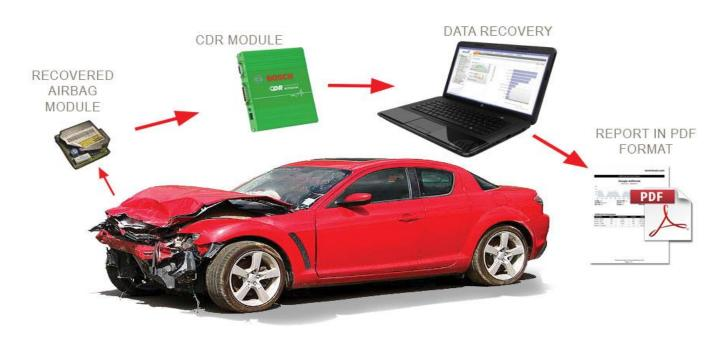
An event data recorder (EDR), similar to an accident data recorder (ADR) sometimes referred to informally as an automotive black box is a device installed in some automobiles to record information related to traffic collisions.
