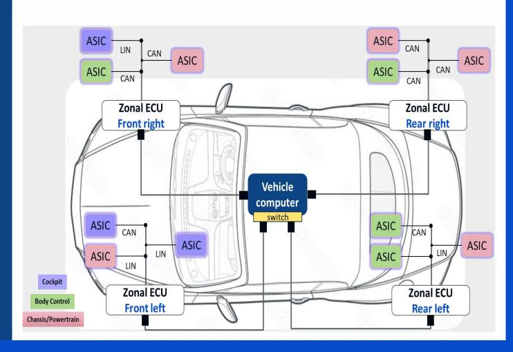
Operates on hardware logic | Do not require firmware | Diagnostics enabled
