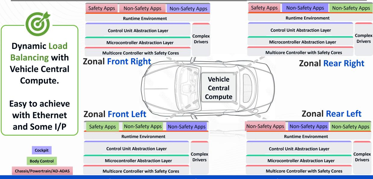
Manage diverse applications | Shared infrastructure | Enhance modularity | Reduce wiring complexity
